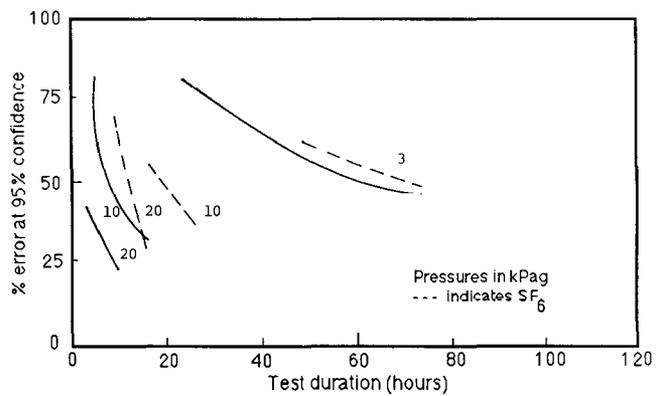
Figure 5 Test error for a target leak rate of 5% per day.
