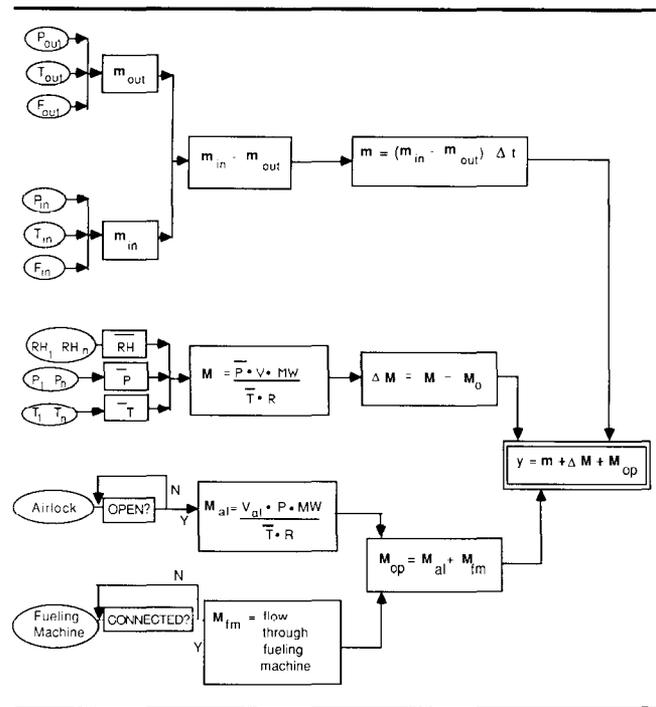
Figure 2 Flow chart of leak rate calculations.
