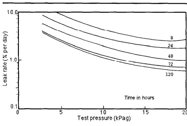
Figure 8 Minimum detectable leak rate at 50% error.
