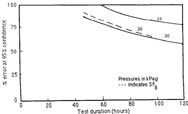
Figure 3 Test error for a target leak rate of 0.5% per day.
