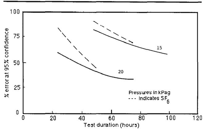
Figure 4 Test error for a target leak rate of 1% per day.
