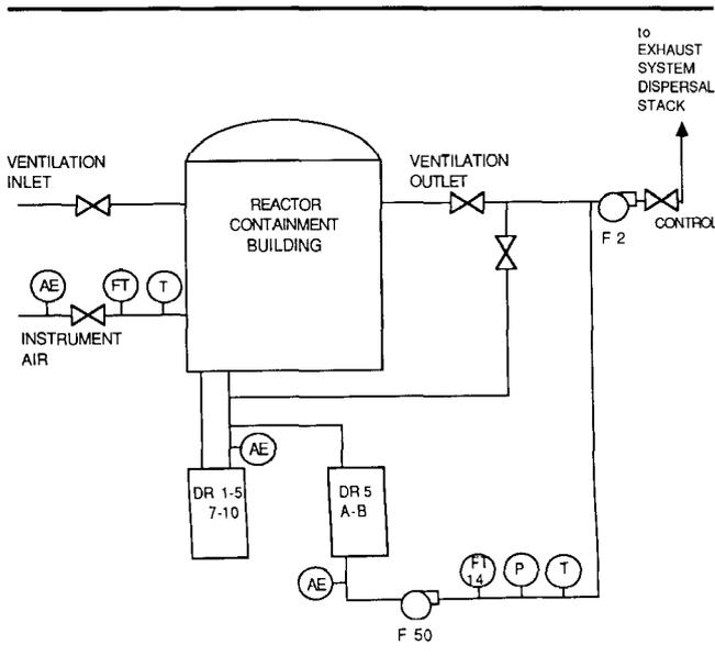
Figure 1 Leak test set up.
