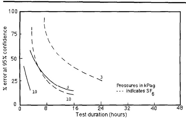
Figure 7 Test error for a target leak rate of 24% per day.
